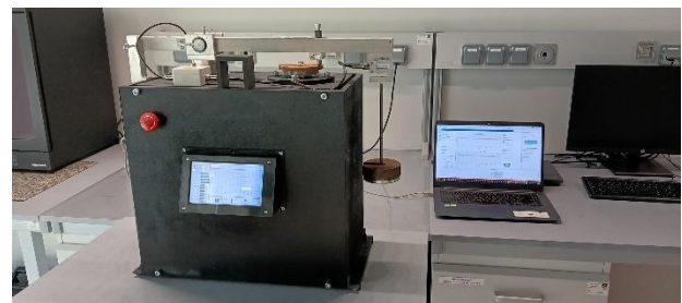
Figure 4. Appearance of the tribometer in a fully assembled state
