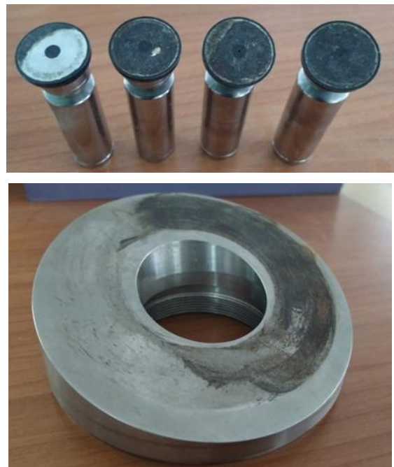
Figure 6. The wear of swash plate and slipper
