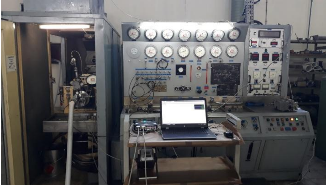
Figure 4. The test pump installed on the test stand
