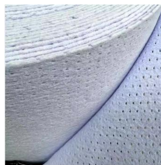
Figure 3. Coremat XI 3 mm [27] [28]
