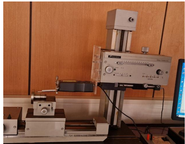
Figure 3. Surface roughness testing on the profilometer
