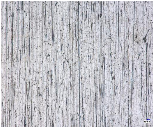
Figure 9. Surface of specimen made of 38GSA steel after friction in soil abrasive compound with a pH of 7.2, magnification: 500x.
