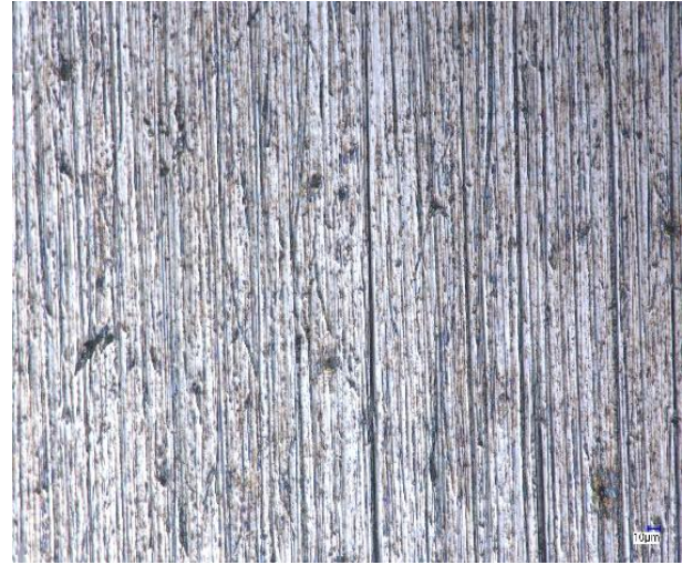
Figure 11. Surface area of the Hardox 500 steel specimen after friction in soil abrasive compound with a pH of 7.2, magnification: 500x.
