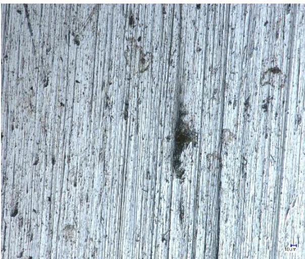
Figure 10. Surface area of the Hardox 500 steel specimen after friction in a soil abrasive compound with an abrasion factor of 3.8, magnification: 500x.
