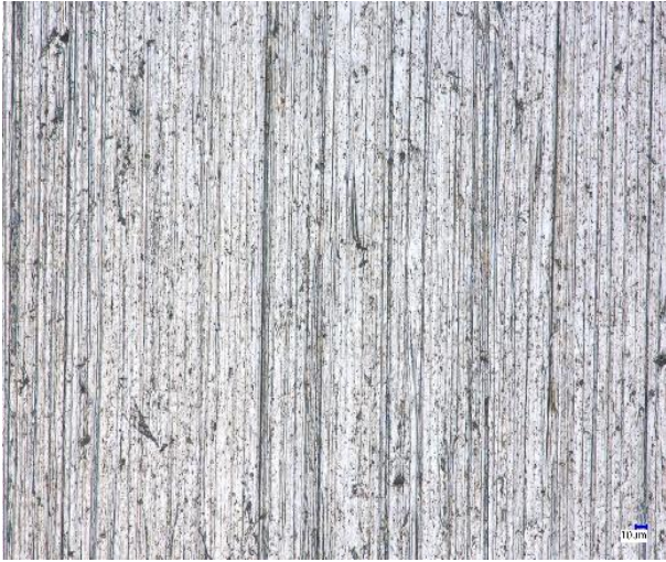
Figure 8. Surface of specimen made of 38GSA steel after friction in soil abrasive compound with a pH of 3.8, magnification: 500x.
