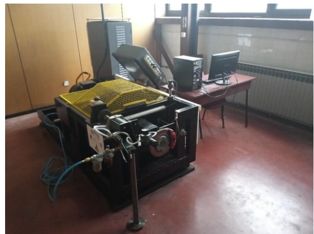
Figure 1. The test rig for the laboratory investigations – BRAKE DYNO 2020
