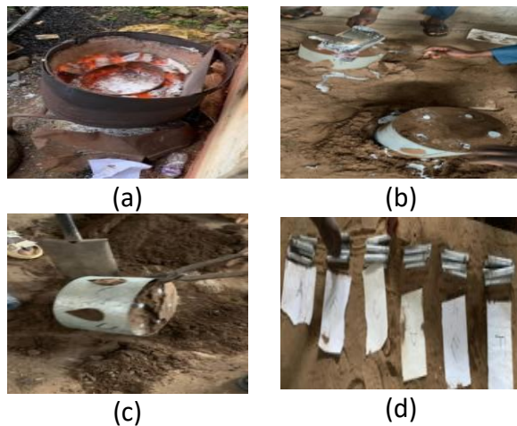
Figure 3. Melting (a) pouring and solidifying (b) shaking out (c) and cast AlSiMg alloy sample (d)
