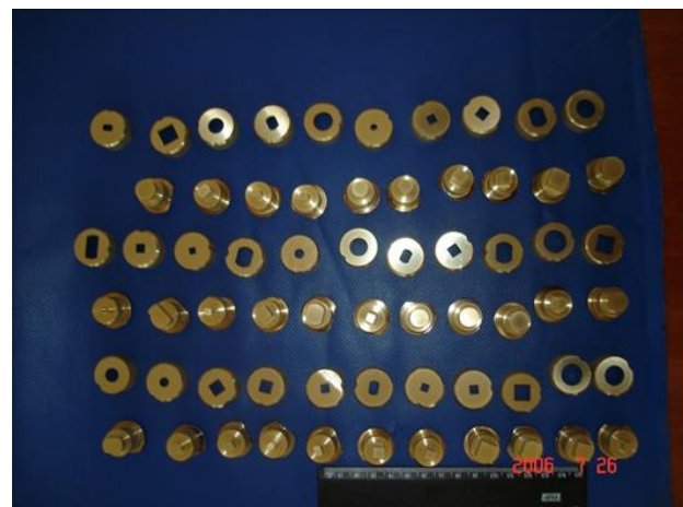
Figure 7. Multitools punching tool with hardening nanocoatings
