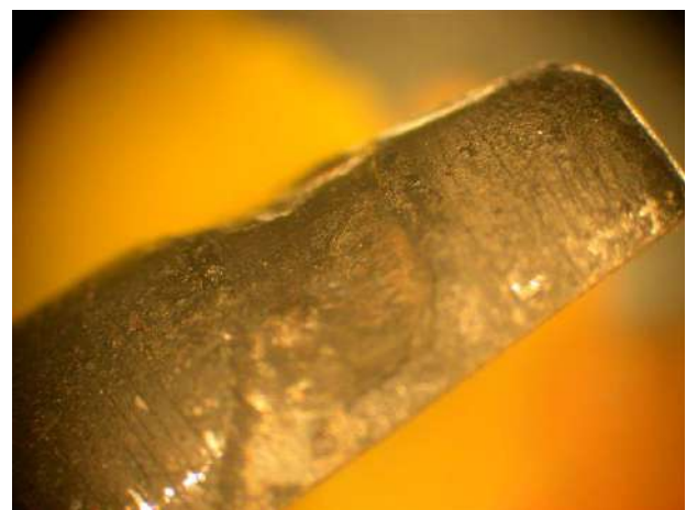
Figure 3. CrN core pin after 14,000 cycles
