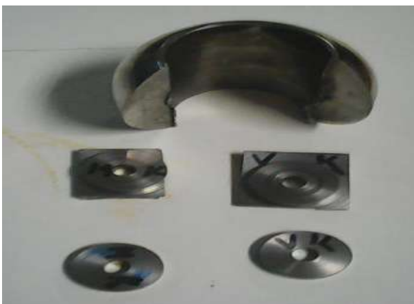
Figure 6. The process of making discs of selected material from the sphere in exploitation
