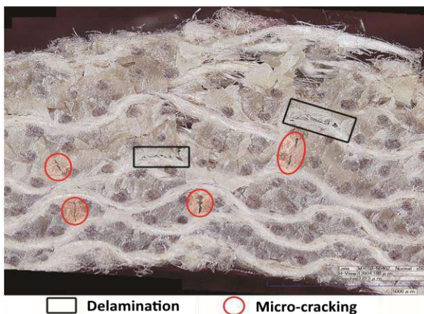
Figure 8. Micrograph of a specimen after aging, showing structural defects
