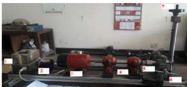
Figure 2. Experimental setup for fatigue test
