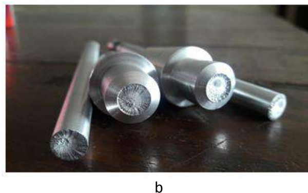
Figure 3. Fretting arrangement (a) and fractured specimens in this experiment (b)
