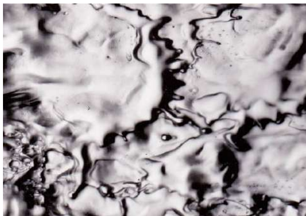
Figure 2. General View of coating from electrode P25 - I = 14.4 A, T_i = 12\mu s C = 1\mu F , \tau = 0.1
