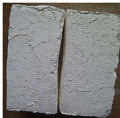
Figure 11: Porous Ceramic with HDPE as pore former showing micro cracks.
