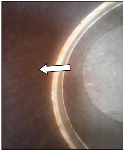
Figure 4. Enlarged part of the samples of metal balls. The body of valve and PTFE sealing ring (lost contact geometry due of exploitation process)
