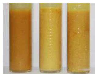
Figure 2. Photograph of mixture ISO VG-220 with 5 % synthetic, semi-synthetic and oil emulsion, after 10 minutes of standstill
