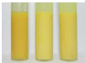
Figure 1. Photograph of mixture ISO VG-68 with 5 % synthetic, semi-synthetic and oil emulsion, after 10 minutes of standstill
