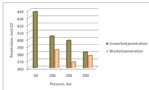
Figure 7. Unworked/worked penetration according to pressure
