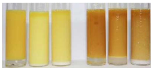
Figure 3. Photograph of mixture ISO VG-68 (left) and VG-220 (right) with 5 % synthetic, semi-synthetic and oil emulsion, after one hour of standstill
