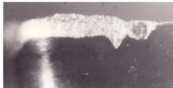
d) Flank wear of uncoated tools Cutting speed V 25m/min, f 0.37mm/rpm, cutting time 40 min
