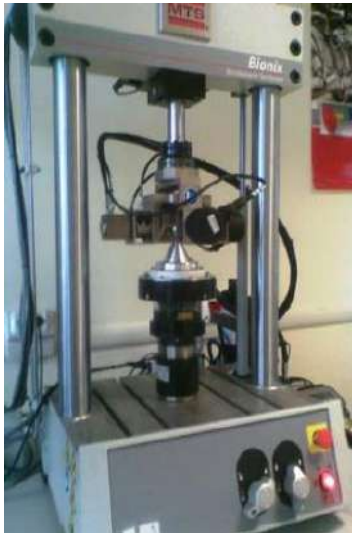
Figure 2. MTS Bionix servo-hydraulic multiaxial dynamic testing machine, equipped with system for testing the hip implants
