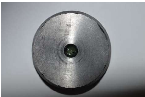
Figure 5. Textured plain bearing sample
