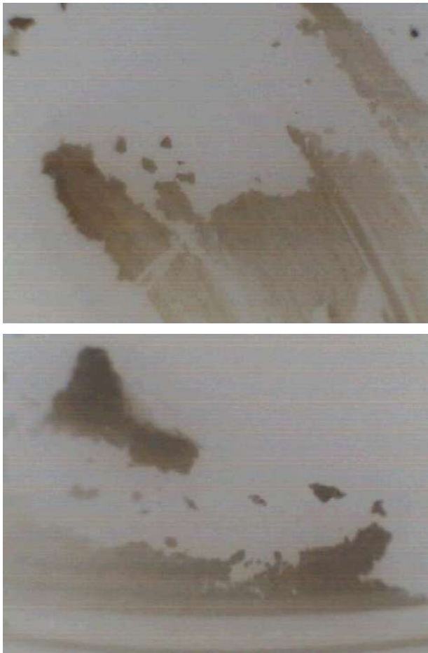
Figure 5. Photographs of fluoropolymer surface after the experiment (the tribopair fluoropolymer – steel 100CrMn6, magnification is 88x)
