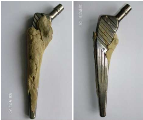
Figure 10. The sides of the cemented stem prosthesis together with a part of the cement mantle, extracted after 2450000 cycles of fatigue test, from Instron® device
