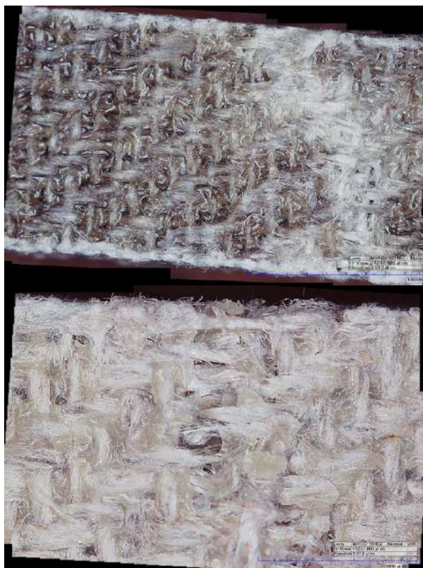
Figure 7. Micrographs of composite surfaces, before (a) and after (b) the aging, showing the effect of embrittlement
